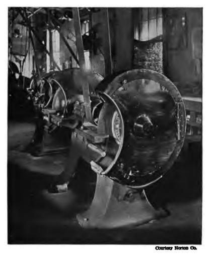
Closed Type of Protection Hood on Grinding Wheel Floor Stand. Hoods connected with a dust exhaust system.
